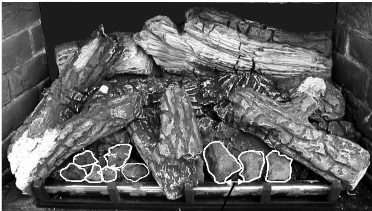
Add Large Chunk Coals behind front burner and on Logs "C" and "D" surfaces. Space Coal Chunks apart at least 1/4" where they touch the Front Burner to allow upward flow paths for Front Burner Flames.
